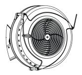
2. Remove the outer flywheel housing, while keeping the mesh strip in place in the inner housing.
