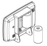
Install 2 x D cell batteries.
